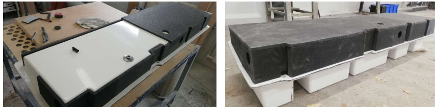
Custom made glass fiber reinforced grey water tank
