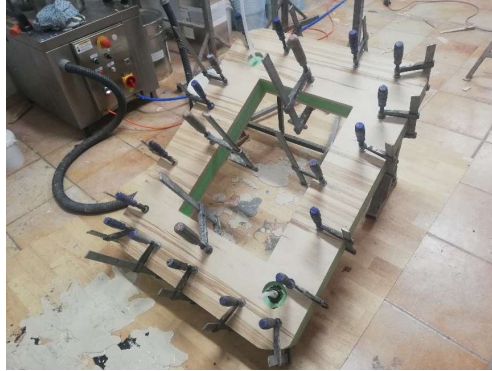
Reactive injection moulding of door window frame
