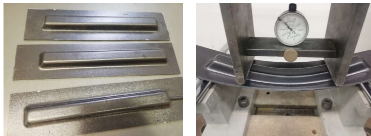
Specimen geometry, and 4-point bending tests of specimens
