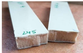
Failure of PVC cored sandwich material made by reactive injection moulding (RIM): skin breaking and skin compression buckling
